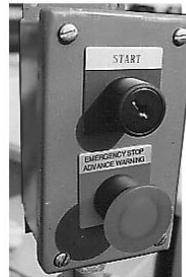
▼ The RJ-225 Ultra features an advanced, simplified control system with 2 button operation. It is key-operated and fully automatic. The heavy duty push button controls are contained in a weather-proof NEMA 4 enclosure. Connected to the power pack with 13' of sealtite, the controls can be located for operator convenience.
